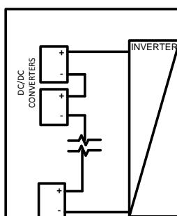
IF DC/DC CONVERTERS ARE USED, THEY ARE RUN IN SERIES (FIXED SOURCE CIRCUIT VOLTAGE DC/DC CONVERTERS)
